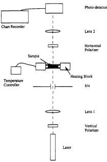
Figure 1. Schematic of the birefringence apparatus used to determine the ODT of the block copolymer solutions.
